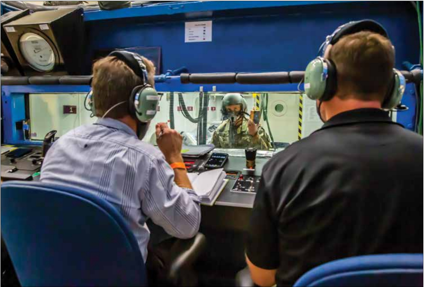
The U.S. Army Aeromedical Research Laboratory collaborates with the U.S. Army School of Army Aviation Medicine to conduct testing inside their man-rated altitude chamber. The goal of this effort was to test three patient isolation units (PIUs) to determine if they will operate correctly when exposed to simulated altitudes from ground level up to 18,000 feet. (Credit: Scott C. Childress)
