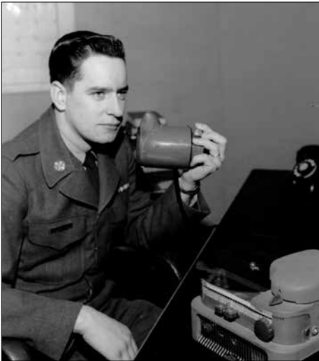
In this April 1958 photograph, Specialist Two Gilbert E. Kaschmeier, a court reporter for the Judge Advocate Section, US Army Garrison, Regional Camp Zama, Japan, demonstrates a “stenomask.” With this device, he can record every word and describe every gesture during court or board proceedings, as rapidly as 420 words a minute.
